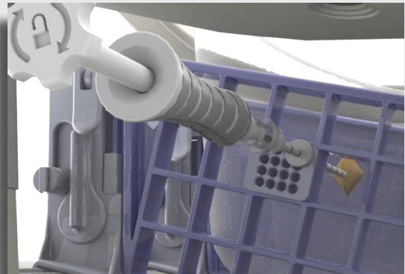
4. Remove adapter from applicator and deploy marker
